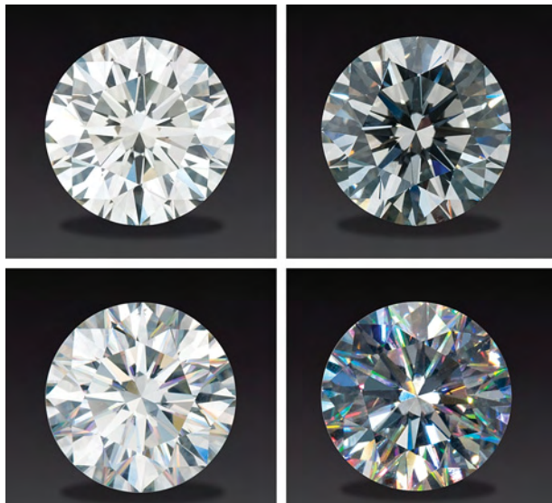
Figure 13. This 2.30 ct diamond originally had a GIA cut grade of Excellent, as shown here in diffused light (top left) and spot lighting (top right). In both environments, there is little fire. After processing with pattern C, it looks much the same in diffused light (bottom left) but has a more dynamic face-up appearance in spot lighting (bottom right). Courtesy of Bob Lynn, Lynn's Jewelry Studio, Ventura, Calif.; photos by Robert Weldon.
