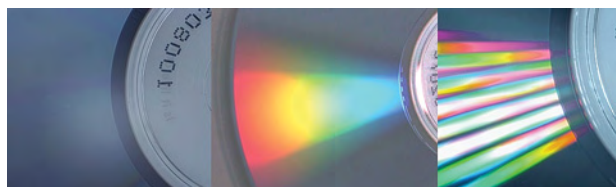
Figure 2. Under diffused lighting (left), the diffraction grating formed by lines on the surface of a compact disc (6,250 lines per centimeter) very faintly separates white light into spectral colors. Under spot lighting (center), the same grating separates a single spot light source into distinct spectral colors, like those in a rainbow. Under an array of spot lighting (right), it separates multiple spot light sources into a myriad of distinct spectral colors. Composite photo by A. Gilbertson.
