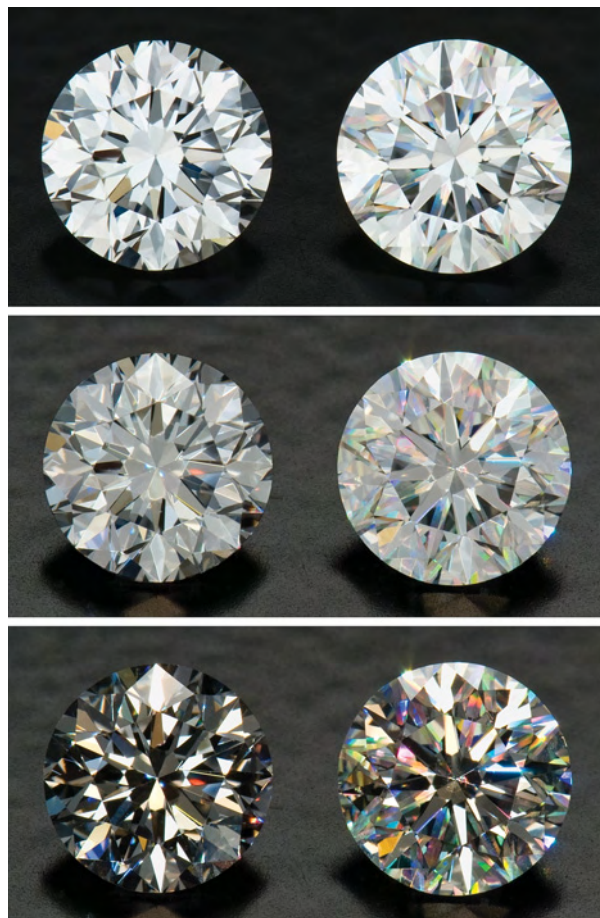
Figure 14. These two diamonds of similar proportions, one cut conventionally (RD01, left) and the other with pattern C (no. 32, right), are shown in three lighting environments: diffused (top), mixed (center), and spot lighting (bottom). When spot lighting is substantial, careful placement of the diffraction grating can improve the appearance of certain diamonds by making them more fiery. Photos by Robert Weldon.
